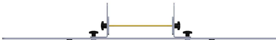
Abb. 2: Through Kalibrierstandard Fig. 2: Through calibration standard
