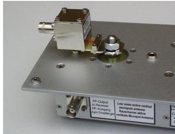
Fig. 10: Combination of matching unit and calibration adapter
